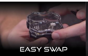
Remove the lens using a small screwdriver or trim tool, and simply snap your new lens in its place!
