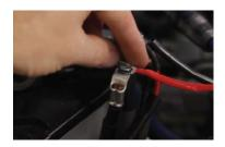
**6.** Connect the red power wire © to the positive terminal on the battery.
