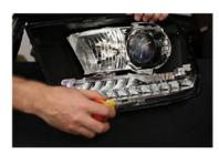
1. Access the factory LED panels by removing the screws holding the turn signal assembly in place. Remove the chrome reflector unit by depressing the clip on the back of the driver.
