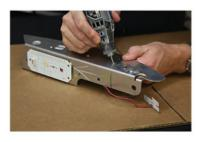
Remove the factory LED board from the metal bracket. Remove the metal rivets holding the LED panel to the turn signal housing with a rotary (Dremel) tool. Panels should fall off.
