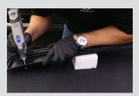
1. Remove the trim panel and take it to a soft working area. Using one of the lightbars, determine where you need to make your cuts on the factory trim panel. Next, use a dremel to cut an opening on both sides of the panel.
