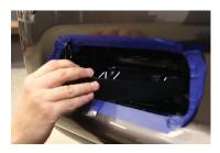
**4.** Feed your lightbar bracket through the opening in the bumper, looping the ends around the bolts on the bumper support. Ensure the longer arm of the bracket is towards the center of the vehicle. Hand-tighten the nuts on the bracket to hold it in place for the next step.
