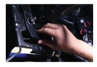
**6.** Adjust the lightbar to your desired height, then fully secure using an 18mm socket.
