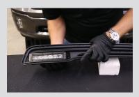
**2.** Ensure your cut is large enough for the lightbar to fit through. Then reinstall the trim panel back onto the truck.
