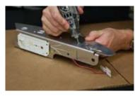
3. Remove the factory LED board from the metal bracket. Remove the metal rivets holding the LED panel to the turn signal housing with a rotary (Dremel) tool. Panels should fall off.
