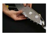
6. Reinstall chrome reflector to housing. Using the alignment notches, be sure to align properly and push gently back into position. Do not use excessive force. If the reflector is misaligned, there is chance of damaging the LEDs. Once complete, replace the torx screws.
