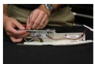
5. Place the new Diode Dynamics LED boards into position on the metal bracket. All holes should align perfectly. Adjust if holes do not line up. Use sturdy twist-ties (included) to fasten boards in place, by passing them through the holes where the metal rivets were. We do not recommend adhesives, as they may fail over time.
