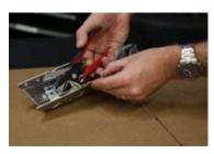
4. Using a wire cutter, cut the wires from factory driver board and remove the panels. If the boards do not easily fall off, make sure to remove any metal burrs that may still be holding them on. You may leave factory driver and sidemarker in place.
