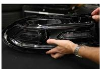
6. Using the alignment tabs, reinstall the black bezel. Once complete, replace the original T-20 screws and headlamp lens. Repeat for other headlamp.
