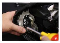
2. Next, remove the two T-20 screws holding the heatsink and black alignment bracket in place. Remove the heatsink and unclip the power connector from the factory board. Remove the two T-15 screws holding the black alignment bracket to the heatsink. Remove the final T-20 screw holding the factory board in place.
