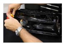
1. First, access the factory board by removing the four T-20 screws holding the black bezel in place. Once removed, pull the bezel out and set it to the side.
