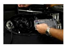
5. Once complete, route the wiring out of the headlamp through the dust cap, sealing any holes that you may create.
