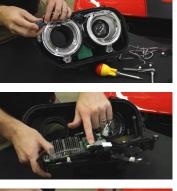
1. After opening the headlights, remove the factory LED panels by removing the screws holding the main bezel in place. Then remove the screws holding each ring and LED panel underneath to the housing.
