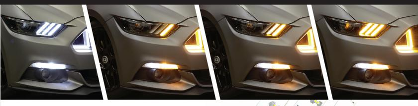
2015-2017 Ford Mustang Switchback DRL LED Boards with sequential turn signal
