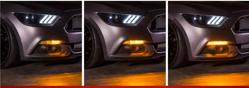
Using the integrated switch, you can program your desired turn signal blink rate.
